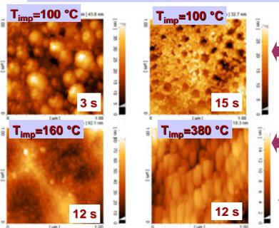
Implanted Ti (at 100 °C): surface oxide layer was removed and there was access to a deeper porous layer.
