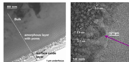
Left: overview, showing the existence of three layers: surface oxide; porous amorphous layer; bulk.
