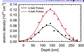
The integral dose of the 2e6 pulses implantation is 0.8 x 10<sup>17</sup> cm<sup>-2</sup>, for the 4e6 pulses it is 1.57 x 10<sup>17</sup> cm<sup>-2</sup>. Measured dose < expected implanted dose (~ 5 x 10<sup>17</sup> cm<sup>-2</sup>).
