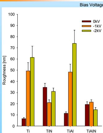
The roughness of all samples was below 100 nm. For coatings without nitrogen the roughness increased with the bias voltage, whereas for coatings with N the roughness was relatively independent from the bias voltage.
